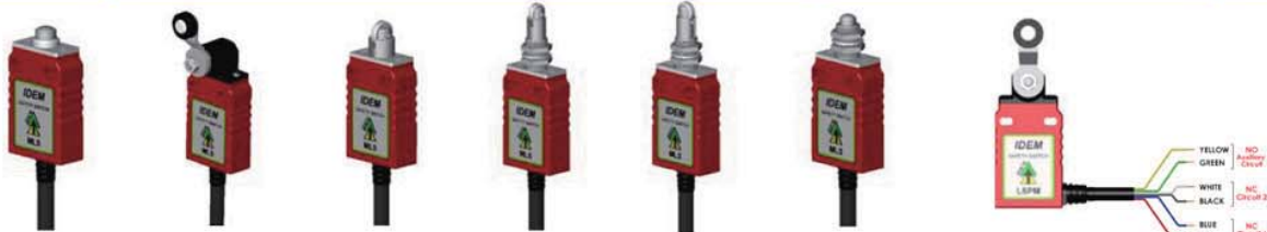
IEC947-5-1 IP67 AC15 A300 240V. 3A. -25 C Max 80 C High Mechanical Life 5,000,000 Rotary or Linear action 2NC 1NO or 1NC 1NO Snap Block Side or bottom cable exit
